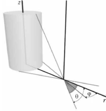
Fig. 2. Arrangement of hot spots of the electrodes.
